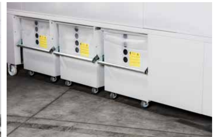
Clamp the chippings container into place
