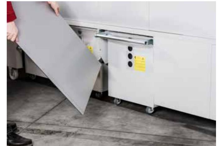
Release the chippings container
